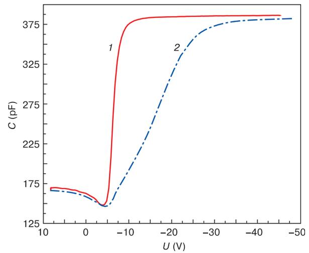
**Figure 1.**  $C-V$  curves of test MOS structure (1) before and (2) after irradiation. Acceleration voltage is of 2.5 keV, beam current of 1 nA and irradiation dose of 15  $\mu\text{Ci}/\text{cm}^2$ .
