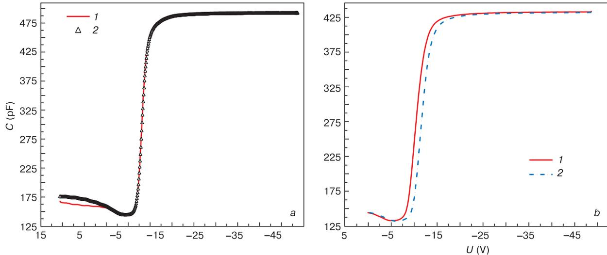
**Figure 3.** Variation of  $C-V$  curves of test MOS structure before electron beam irradiation for application of different bias to metallization (a) +40 V (inversion), (b) -40 V (accumulation), (1) before biasing and (2) after biasing for 15 min.
