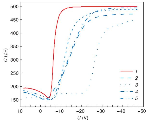
**Figure 4.** Variation of  $C-V$  curves of test MOS structure (1) before irradiation and (2–5) after irradiation with different bias: (2) +10 V, (3) 0, (4) -10 V and (5) -20 V. Irradiation dose:  $20 \mu\text{C}/\text{cm}^2$ .
