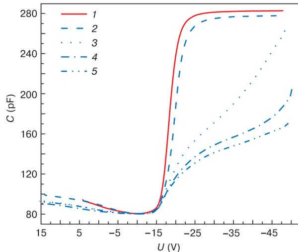
**Figure 2.**  $C-V$  curve variation for different irradiation doses: (1) before irradiation and (2–5) irradiation with doses of 10, 20, 25 and 30  $\mu\text{Ci}$ .
