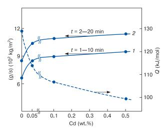
**Figure 4.** Isochrones of oxidation (723 K) of the aluminum conductive alloy E-AlMgSi (Aldrey) doped with cadmium
