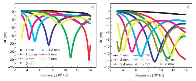
**Figure 9.** Frequency dependences of reflection coefficient of nanocomposites for different metal content ratios in precursor Fe : Co : Al: (a) 40 : 40 : 20; (b) 35 : 35 : 30.
