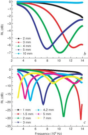
**Figure 7.** Frequency dependences of reflection coefficient of FeCoAl/C nanocomposites synthesized at different temperatures  $T_{\text{synth}}$  °C: (*a*) 500, (*b*) 600 and (*c*) 700.
