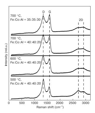
Figure 3. Raman spectra of FeCoAl/C nanocomposites synthesized at different temperatures and metal ratios.
