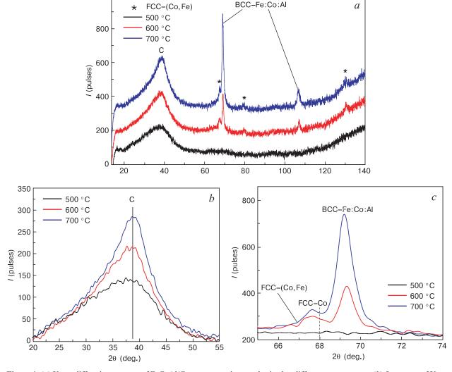
**Figure 1.** (*a*) X-ray diffraction patterns of FeCoAl/C nanocomposites synthesized at different temperatures, (*b*) fragments of X-ray patterns in the vicinity of the angular range for the graphite (002) plane and (*c*) for the (111) and (110) planes of the metallic alloy.
