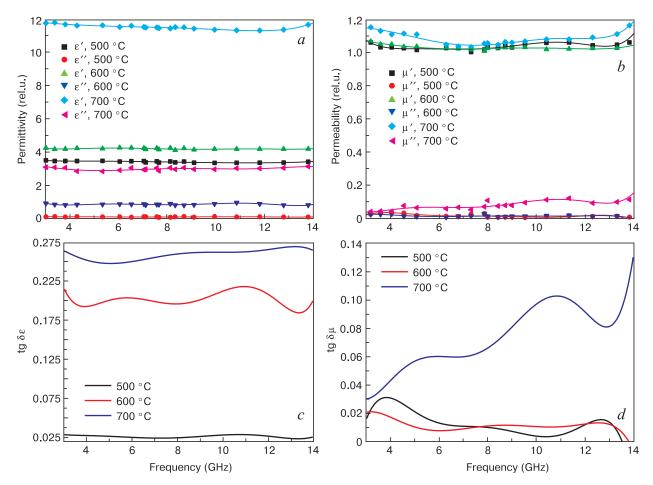
**Figure 5.** Frequency dependences of (*a*) complex permittivity and (*b*) permeability and tangents of (*c*) dielectric and (*d*) magnetic loss for different FeCoAl/C nanocomposite synthesis temperatures.
