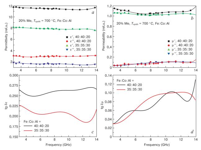
**Figure 8.** Frequency dependences of (*a*) complex permittivity and (*b*) permeability and tangents of (*c*) dielectric and (*d*) magnetic loss for different metal ratios in precursor.
