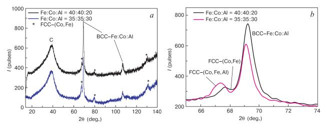
**Figure 2.** (*a*) X-ray diffraction patterns of nanocomposites and (*b*) fragment of X-ray diffraction pattern near  $2\theta = 65^{\circ} \div 74^{\circ}$  for different ratio of metal weights Fe : Co : Al ( $T_{\text{synth}} = 700 \text{ °C}$ ).
