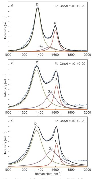
**Figure 4.** Deconvolution of Raman spectra of FeCoAl/C nanocomposites synthesized at different temperatures (°C): (*a*) 500; (*b*) 600; (*c*) 700.
