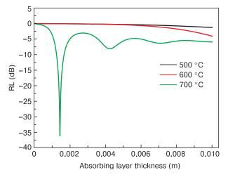
Figure 6. Optimization of absorbing layer thickness.
