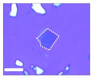
**Figure 1.** Optical image of the  $WSe_2$  flake. The length of the scale bar is 5  $\mu$ m. Dotted line shows 2D WSe<sub>2</sub> flake.
