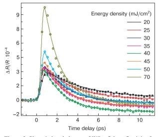
**Figure 2.** Photo-induced change of  $WSe_2$  flake reflectivity for different pump powers. Solid lines – the result of approximation.
