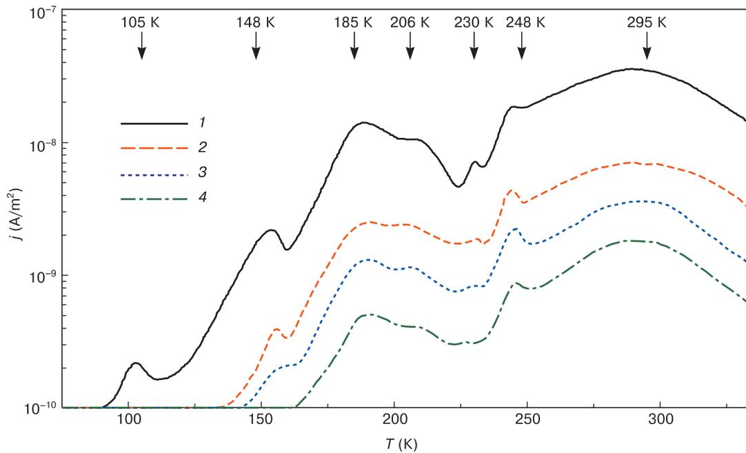
**Figure 8.** Muscovite mica TSD current density as a function of  $E_p$  for  $T_p = 323$  K and  $t_p = 10$  min for  $E_p$  field magnitudes, V/m: (1)  $5 \times 10^6$ ; (2)  $10^6$ ; (3)  $5 \times 10^5$ , (4)  $2 \times 10^5$ .
