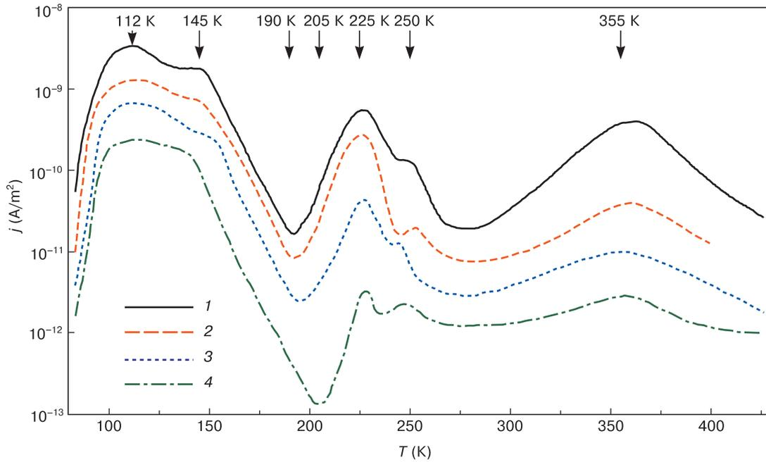
**Figure 4.** TSD current density of  $\alpha$ -LiIO<sub>3</sub> single crystals along [0001] axis as a function of  $E_p$  for  $T_p = 323$  K,  $t_p = 10$  min,  $d = 0.7$  mm, electrode diameter 25 mm and  $E_p$  field magnitudes, V/m: (1)  $8.5 \times 10^5$ ; (2)  $4 \times 10^5$ ; (3)  $2 \times 10^5$ ; (4)  $5 \times 10^4$ .
