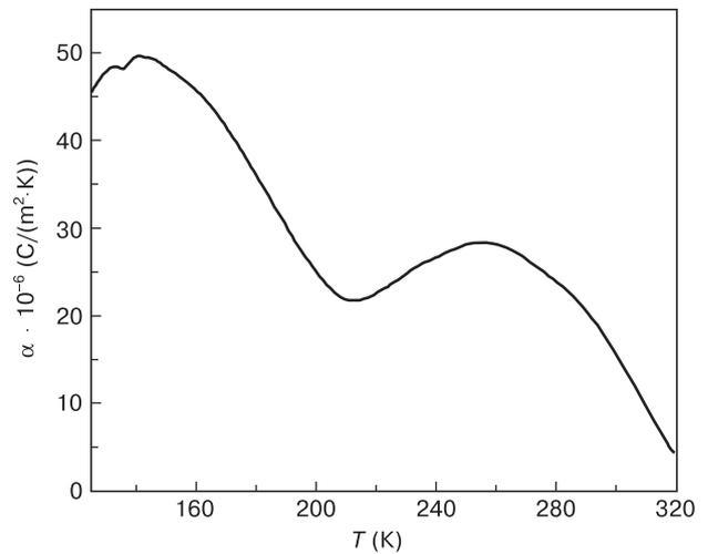
**Figure 5.** Temperature dependence of pyroelectric effect in  $\alpha$ -LiIO<sub>3</sub> single crystals [12].
