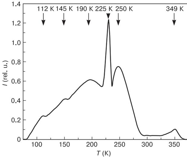
**Figure 6.** Thermally stimulated luminescence spectrum of  $\alpha$ -LiIO<sub>3</sub> crystals:  $t_p = 1$  h,  $U = 15$  kV,  $T_p = 80$  K. Irradiation on URS-2.0 X-ray apparatus.  $t_p$ ,  $U$  and  $T_p$  are polarization time, voltage and temperature, respectively.
