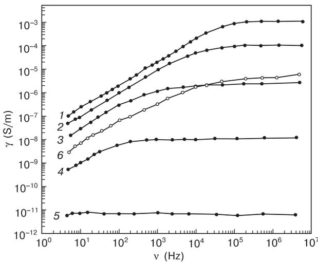
**Figure 9.** Frequency dependence of electrical conductivity of  $\alpha$ -LiIO<sub>3</sub> crystals at temperatures of (1) 297, (2) 265, (3) 229, (4) 183 and (5) 125 K along the optical axis and (6) 297 K perpendicular to the optical axis.
