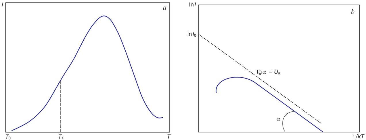
**Figure 1.** Defect parameter determination from TSD spectra with the Garlick–Gibson method: (a) TSD temperature dependence in linear heating mode, (b) TSD curve in Arrhenius coordinates with initial rise section.
