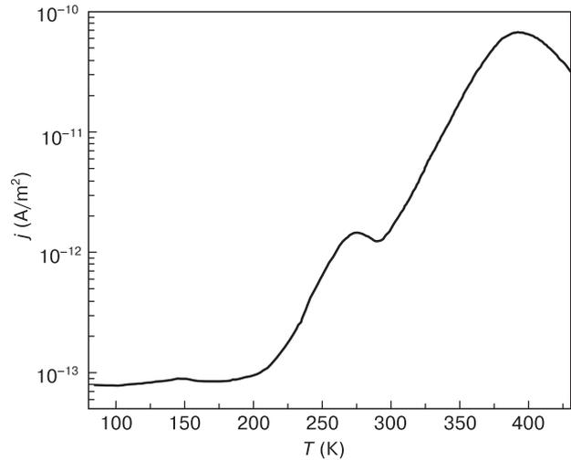
**Figure 7.** TSD spectrum of  $\alpha$ -LiIO<sub>3</sub> crystals taken perpendicular to the sixth order axis at  $E_p = 4 \times 10^5$  V/m and  $T_p = 376$  K.
