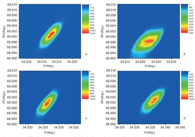
**Figure 1.** X-ray diffraction intensity maps near Si (400) site for Specimens (*a* and *b*) 1 and (*c* and *d*) 3: (a and c) before and (*b* and *d*) after treatmen
