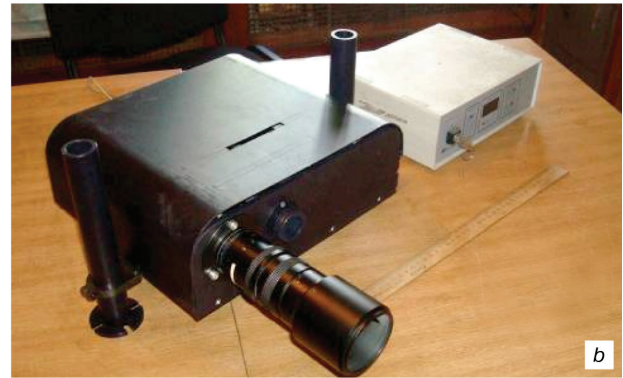
Figure 2. (a) Schematic diagram of experimental setup and (b) general appearance of digital holographic interferometer.
