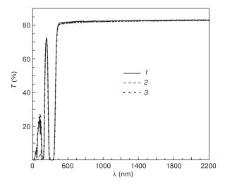
**Figure 1.** Transmittance spectra of (*1*) GAGG : Ce; (*2*) GAGG : Ce,Ca and (*3*) GAGG : Ce,Zr crystals.
