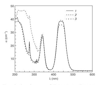
**Figure 2.** Absorption spectra of (*1*) GAGG : Ce; (*2*) GAGG : Ce,Ca and (*3*) GAGG : Ce,Zr crystals.
