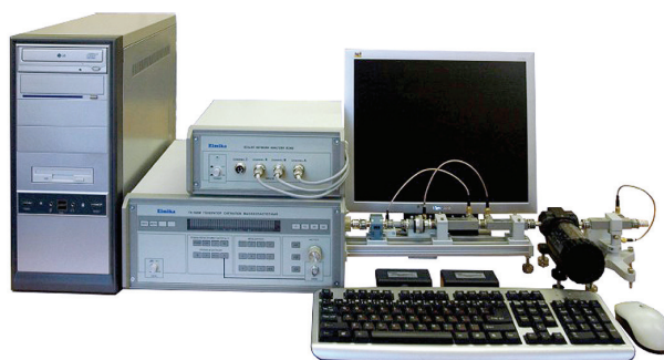
Figure 2. General appearance of R2-124M panoramic voltage standing wave ratio and attenuation meter.
