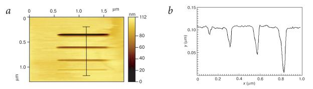
Figure 1. (*a*) SPM image and (*b*) surface profile along the marked line of sample with several grooves formed using (upward) 1, 20, 30 and 100 needle passes.
