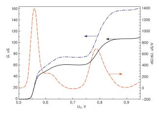
**Figure 3.** Sample conductance *G* (solid curve), channel conductance without allowance for contact resistance (dot-and-dash curve) and dG/dU derivative (dashed curve)) as a function of gate voltage  $U_{c^2}$  used for more accurate quantization step positioning.
