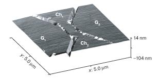
**Figure 2.** SPM image of nanostructure with two  $G_1$  and  $G_2$  controlling side gates and  $Ch_1$ – $Ch_2$  channel.
