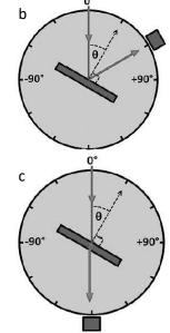
Figure 1. (a) Appearance of the Cary 5000 spectrophotometer with a UMA accessory, (b) specular reflectance measurement experimental setup and (c) transmittance measurement experimental setup.
