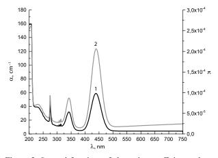
**Figure 3.** Spectral functions of absorption coefficient and extinction coefficient: (1) absorption coefficient and (2) extinction coefficient
