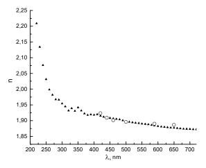
**Figure 5.** Dispersion functions of refractive index obtained using  $(\circ)$  Brewster method and  $(\blacktriangle)$  reflection at low incidence angle close to normal
