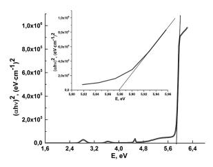
**Figure 4.** Gd<sub>3</sub>Al<sub>2</sub>Ga<sub>3</sub>O<sub>12</sub>: Ce optical band gap determination using Tauc method
