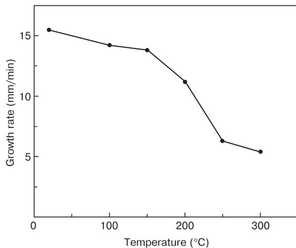
**Figure 3.** SCF deposition rate as a function of substrate temperature
