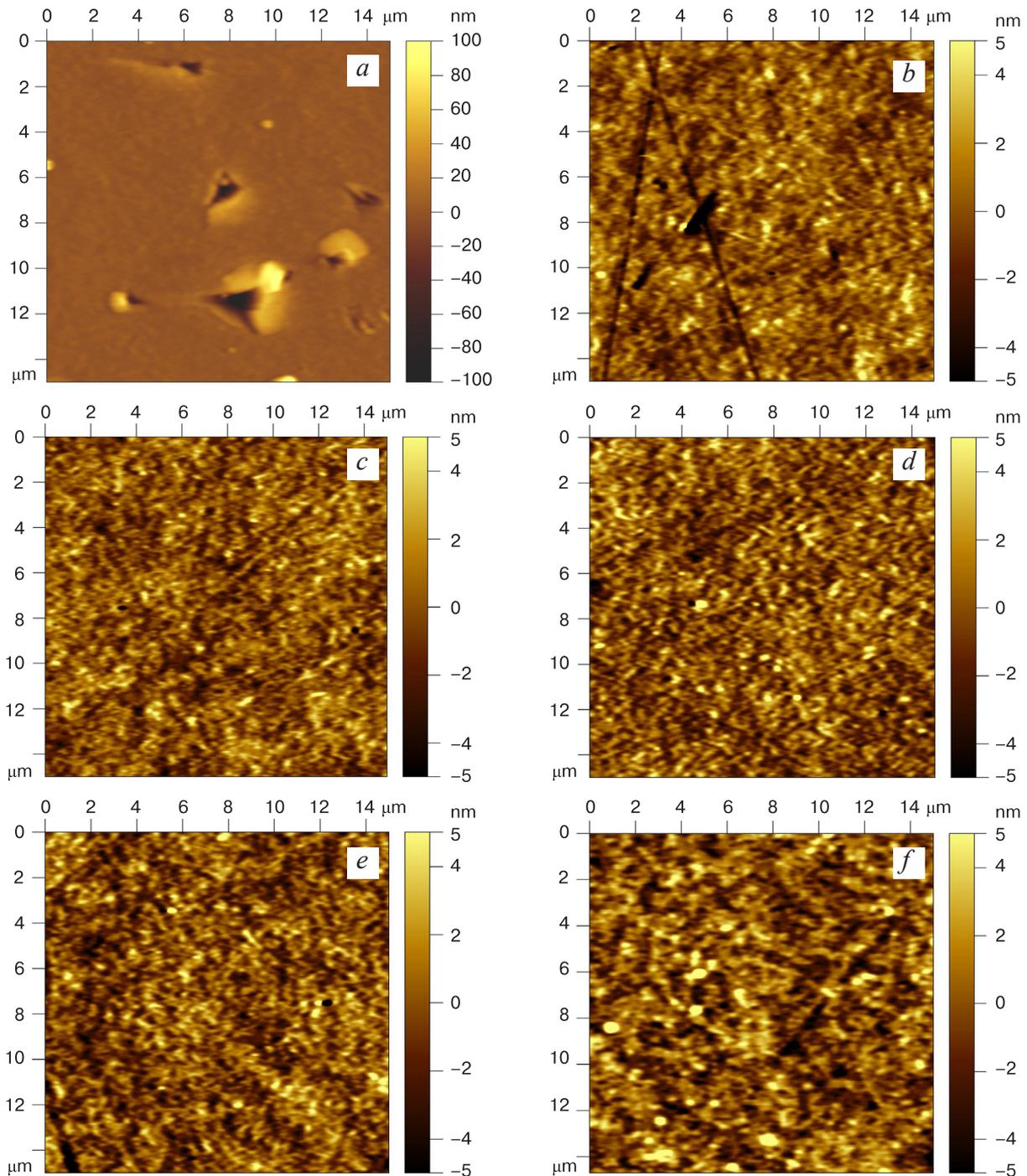
**Figure 2.** Surface images of SCFs grown at different substrate temperatures: (a) room, (b–f) 100, 150, 200, 250 and 300  $^{\circ}\text{C}$ , respectively
