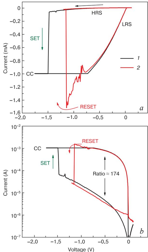
**Figure 8.** Current-voltage characteristics of SCFs: (a) standard and (b) semi-logarithmic coordinates
