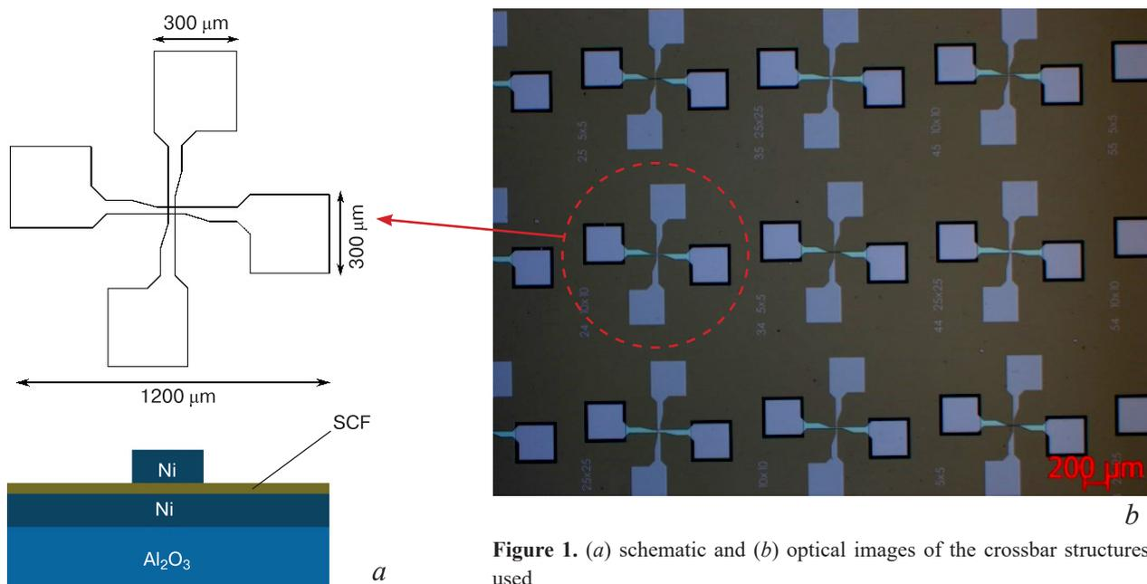
**Figure 1.** (a) schematic and (b) optical images of the crossbar structures used
