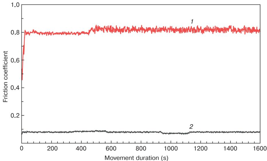
**Figure 5.** Sliding friction coefficients for (1) uncoated Sitall substrate and (2) SCF-coated substrate
