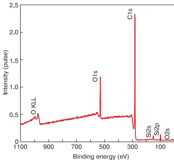
**Figure 6.** Survey XPS spectrum of SCF
