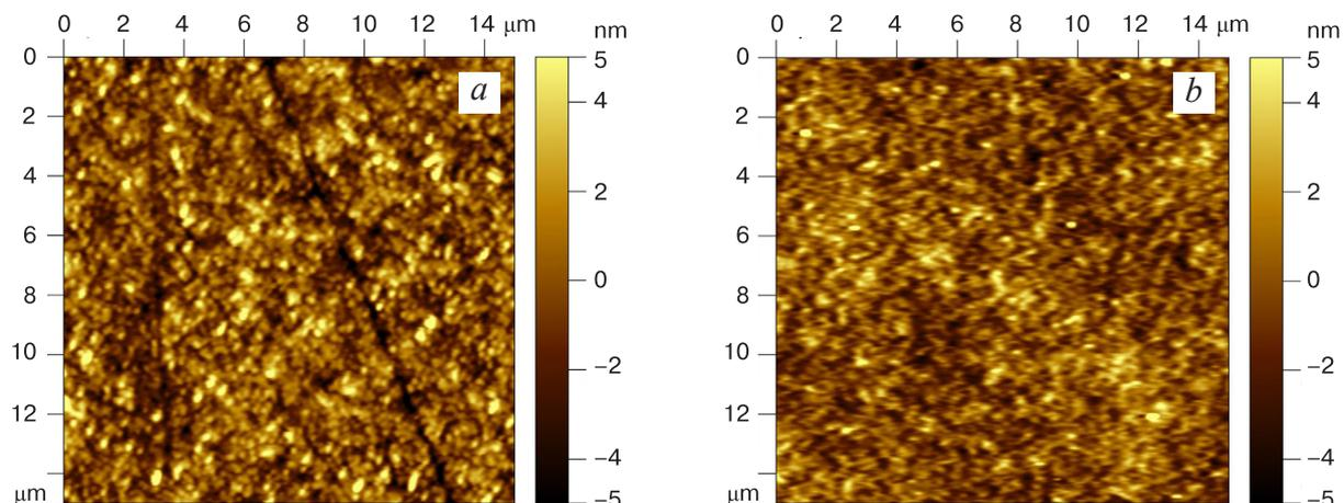
**Figure 4.** Surface roughness of (a) Sitall substrate and (b) synthesized SCF
