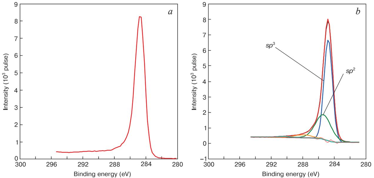
**Figure 7.** XPS spectra of carbon in SCF (a) before and (b) after approximation
