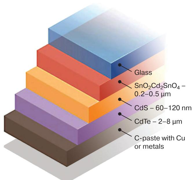
**Figure 1.** Typical CdTe SC structure [9]
