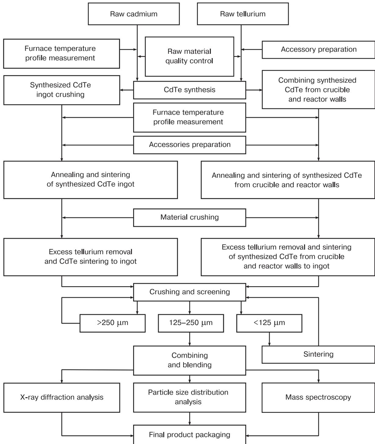
**Figure 3.** CdTe powder process route providing required properties and grain size distribution
