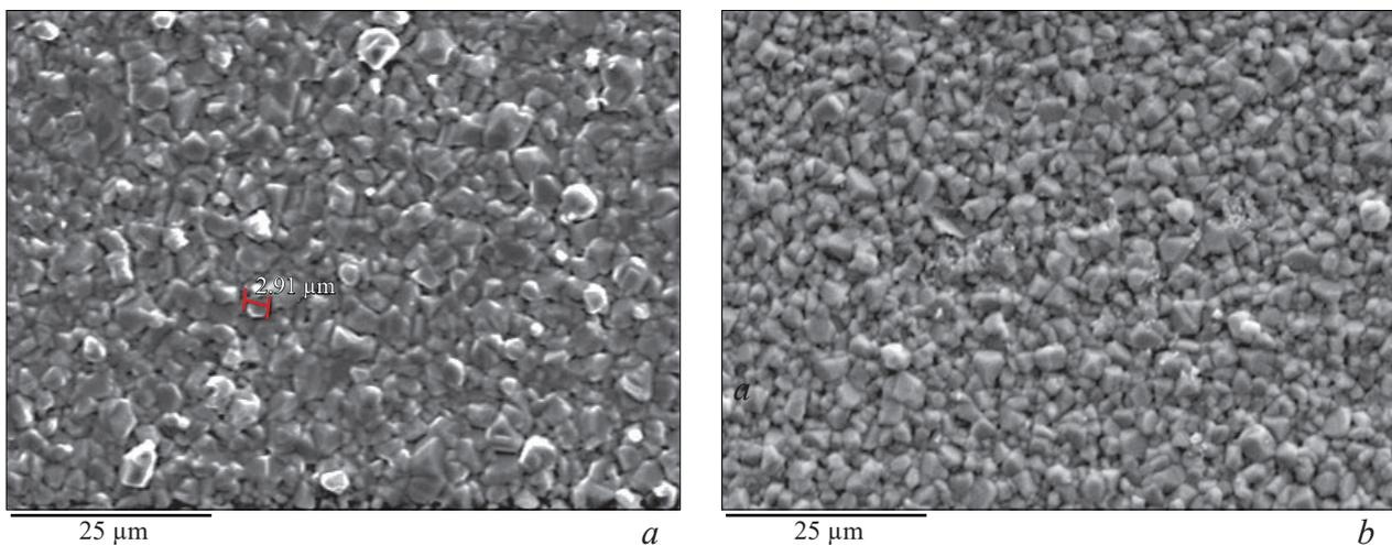
**Figure 2.** SEM morphology of films made from Calyxo powders (a) before and (b) after endurance tests
